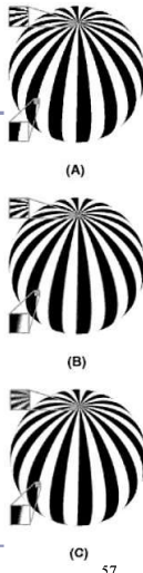
(A) Jagged lines visible in the box function of the procedural stripe texture (B) Fixed-width averaging blurs adjacent samples in texture space; aliasing still occurs at the top, where adjacency in texture space does not align with adjacency in pixel space. (C) Adaptive analytic prefiltering smoothly samples both areas. Image source: Figure 17.4, p. 440, OpenGL Shading Language, Second Edition , Randi Rost, Addison Wesley, 2006. Digital image scanned by Google Books. Original image by Bert Freudenberg, University of Magdeburg, 2002.
